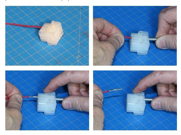
**Step 7** After wires are inserted into connector verify that all the colors line up.
