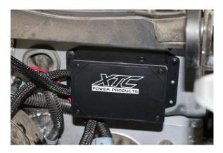
**STEP 2** Mount Fuse box on fire wall, make sure it is mounted where it can be accessed to replace fuses.
