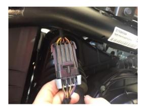
Plug the adapter into both OEM connectors.
